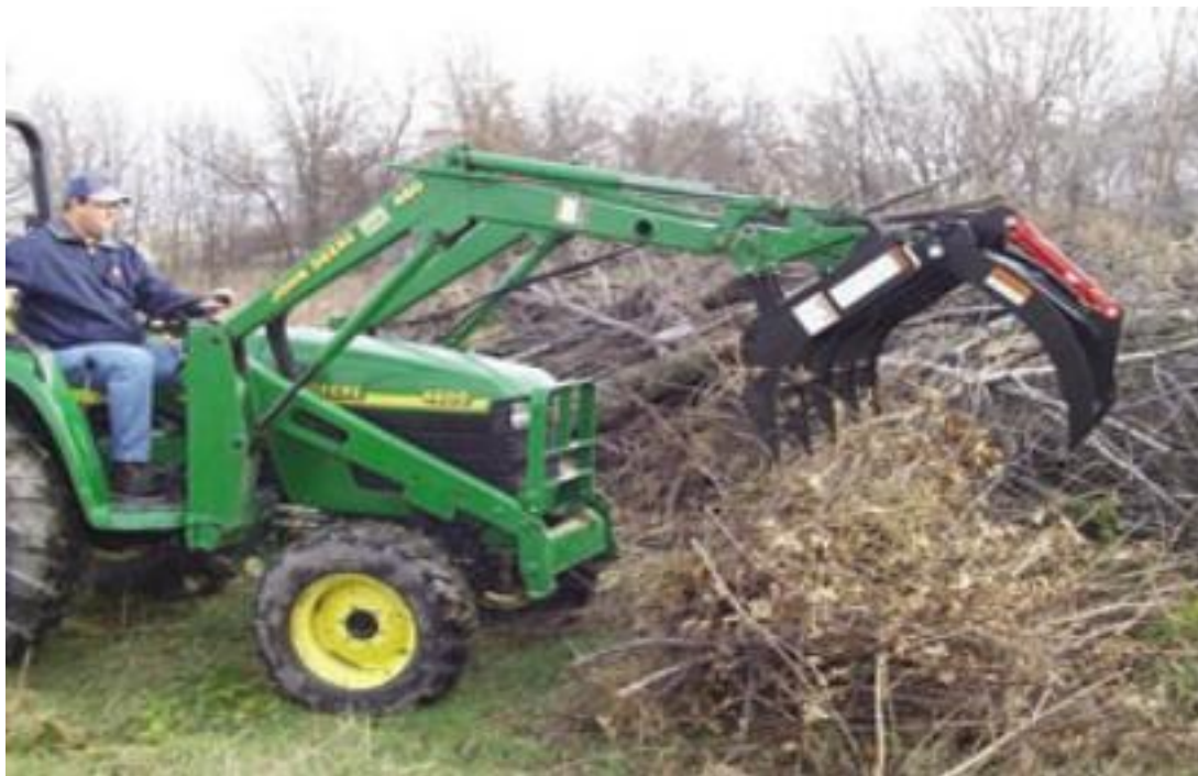
Figure 6: Tractor with attached Material grabber (handler) for loading the cut tree to its trailer.
