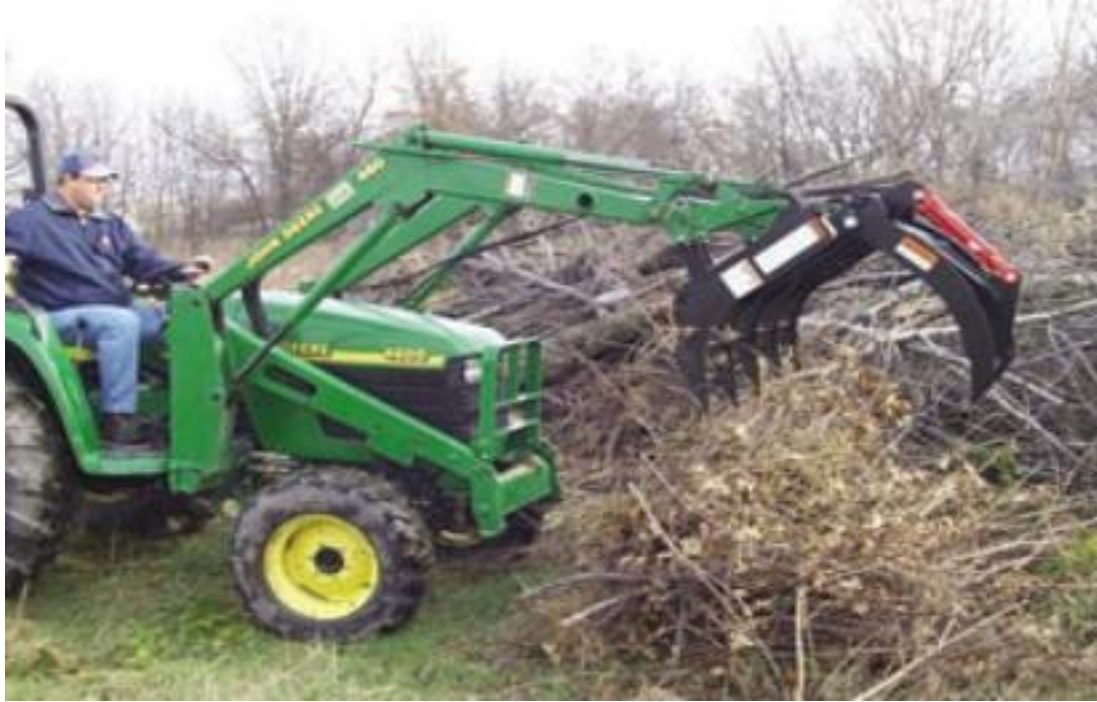
Figure 10: Tractor with attached Material grabber (handler) for pushing the tree to the built-in fork feeder of the tub grinder. 拖拉机带材料抓取器（处理器），用于将树推到桶式碎料器的内置叉式进料器。
