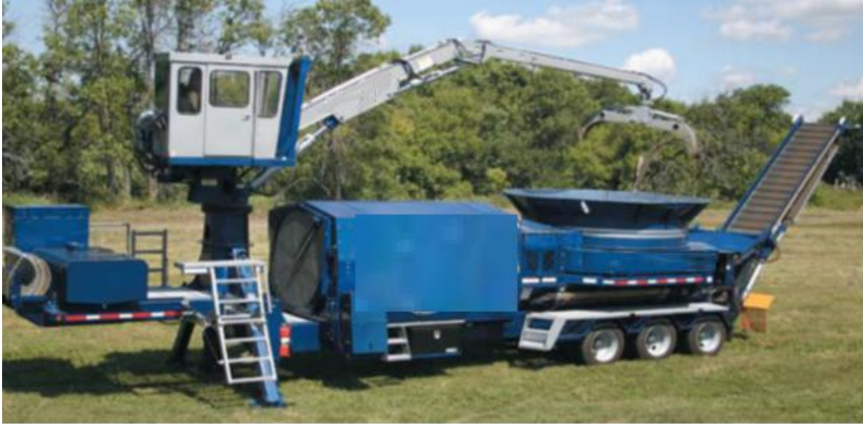
Figure 8: Tub Grinder ready for operation 准备运行的桶式碎料机
