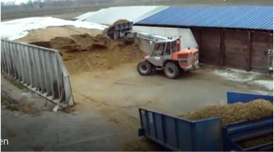
Figure 12: Wheel loader (Mini) loading biomass to the baler 轮式装载机正将料装至打包机上
