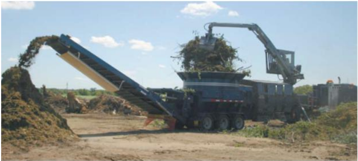
Figure 9: Tub grinder under operation 工作下的桶式碎料机
